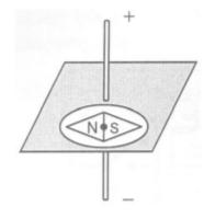
Apply the left hand rule. Have your thumb point up because the electricity is flowing straight (like your thumb) from (-) to (+). Notice that the rest of your fingers point left. This is the direction of the magnetic field in front of the wire. The field is caused by the moving electrons.
